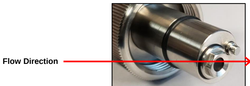
Figure 3.3: Sensor orientation relative to flow direction.
