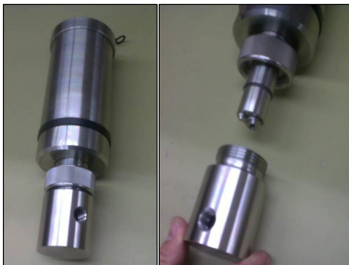
Figure 3.2: Fitting the sensor into the flowcell.
