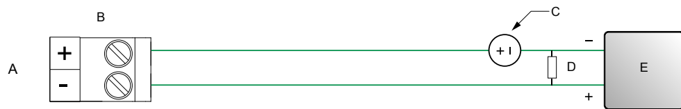
Figure 3-9: Discrete Output wiring (externally powered)
