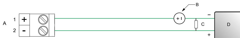
Figure 3-7: Channel A mA/HART output wiring (externally powered)
