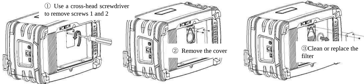
Figure 8- 1 Disassembly of the suction filter
