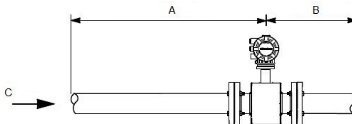
Figure 3-1: Upstream and downstream straight pipe diameters
