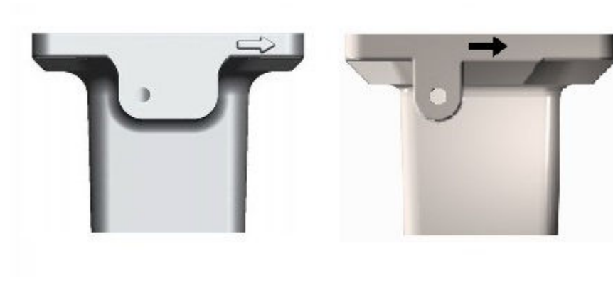
Figure 3-2: Flow direction arrow
