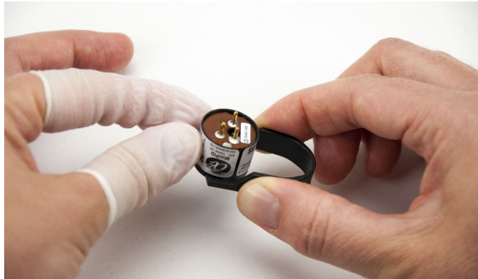
Figure 14: Using Removal Tool
