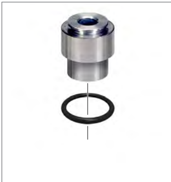
Remove the cylinder o-ring...
