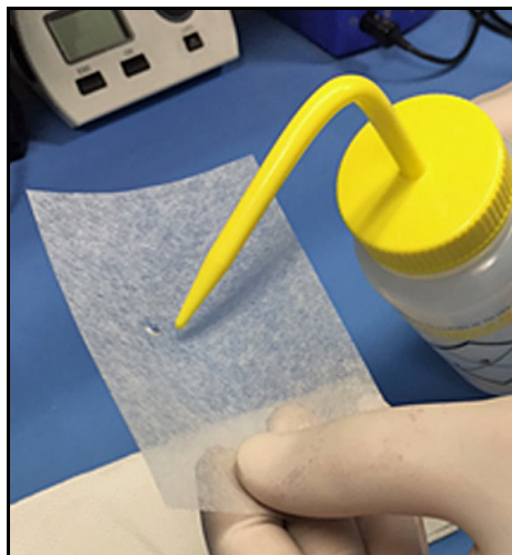
Figure 94: Applying Acetone to Lens Tissue
