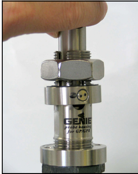
Figure 20: Rotating the Probe
