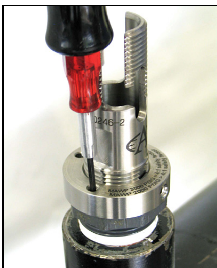
Figure 15: Tightening the Allen Screws
