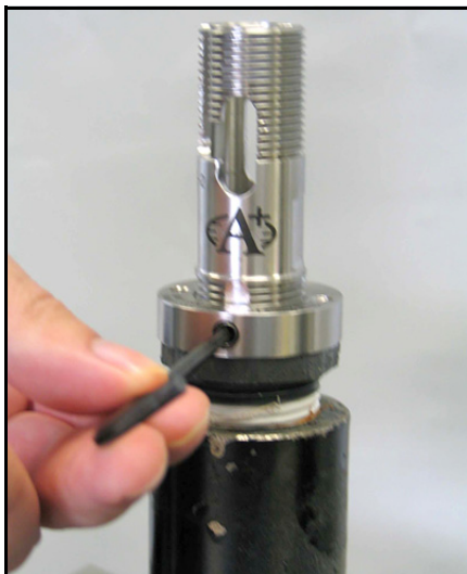
Figure 14: Aligning and Tightening the Allen Screw
