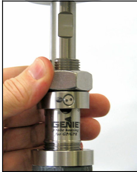
Figure 22: Tightening the Insertion Nut
