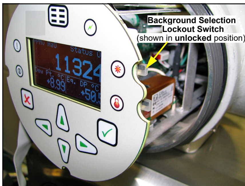
Figure 106: Background Selection Lockout Switch Location
