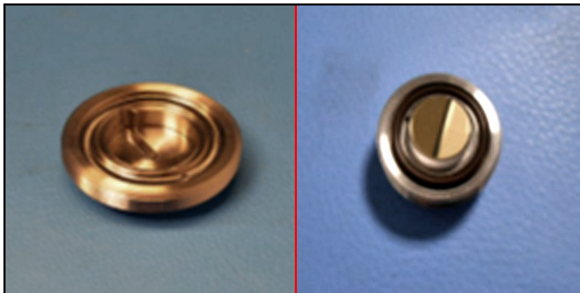
Figure 96: Replacing Cleaned Mirror into End Cap Assembly
