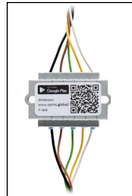
IR app connector: USB programming adaptor incl. terminal block [ACCSMIAC]
