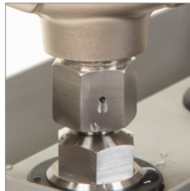
until fluid drips from the CPF weep hole.
