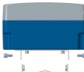
Figure 8: Secure the bracket
