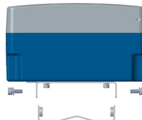
Figure 16: Secure the bracket
