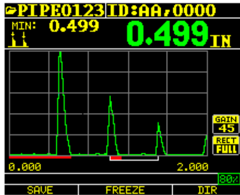
Example of echo to echo with blanking
