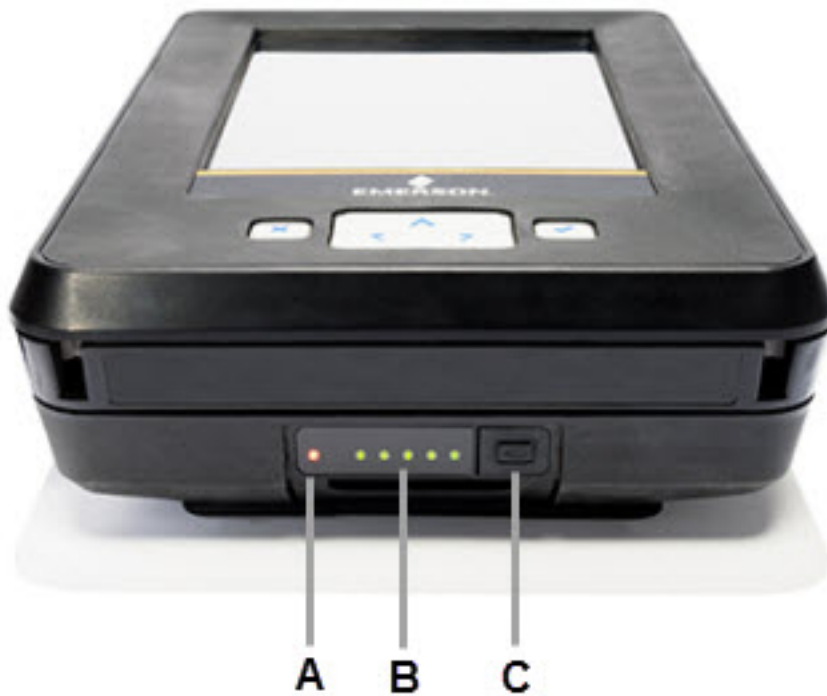
Figure 2-9: LEDs showing approximately 100 percent charge
