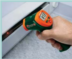
Test for temperature in heating systems
