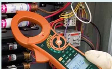
Built-in non-contact Voltage detector with LED alert
