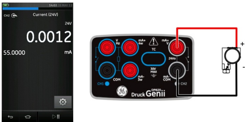
Figure 2-19 Measure current on CH2 with internal loop power (Range: \pm 55\text{mA} )
