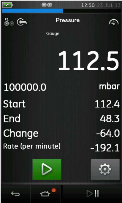
Figure 3-9 Leak Test Example
