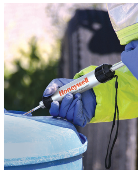
First responder uses Honeywell Colorimetric Tubes and Hand Pump to measure VOC levels inside a barrel.
