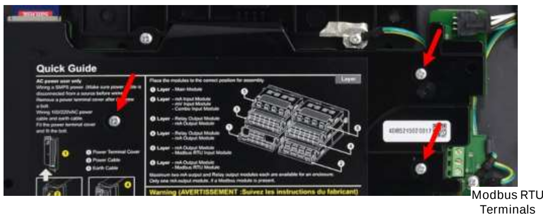
Figure 39. PCB Cover Screws (Arrowed)
