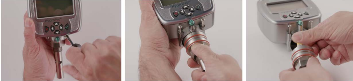
Figure 17: Step-by-step removal of the Hygro II RTE probe from the transmitter
