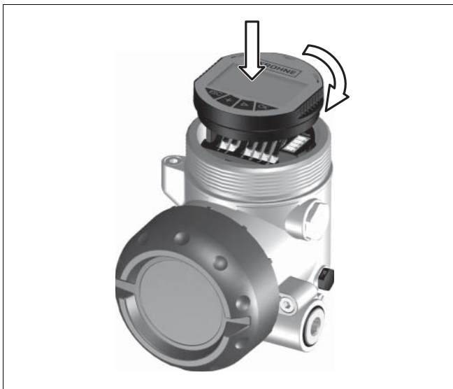
Fig. 20: Installation of the indicating/adjustment module
