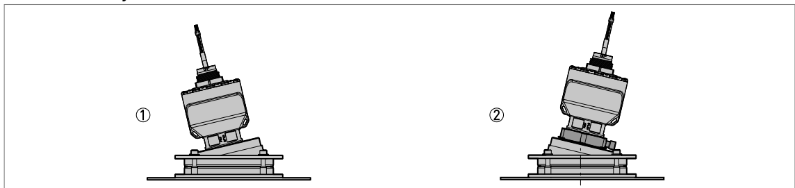
Figure 3-4: Installation of a device with an orientation system (max. tilt 30°)
