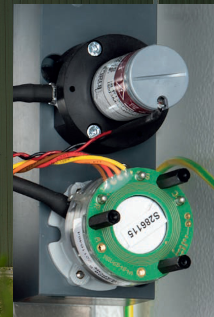
Electrochemical sensors for H 2 S and O 2 measurements
