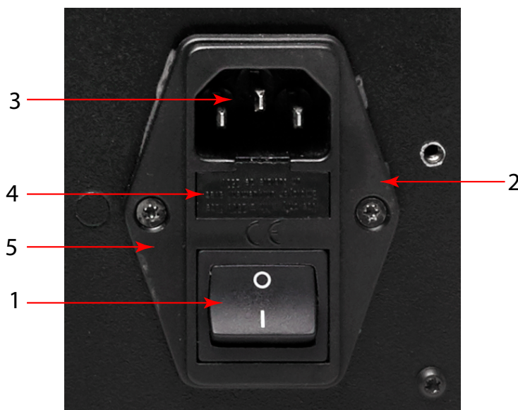
Figure 27 Power Supply Fuse Replacement
