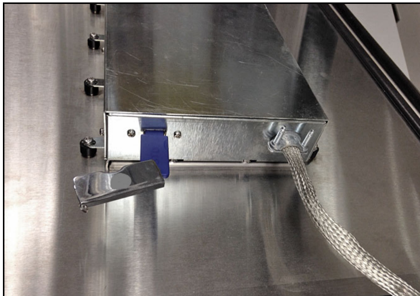
Figure 92: USB Flash Drive Plugged into Chassis Inside the Door
