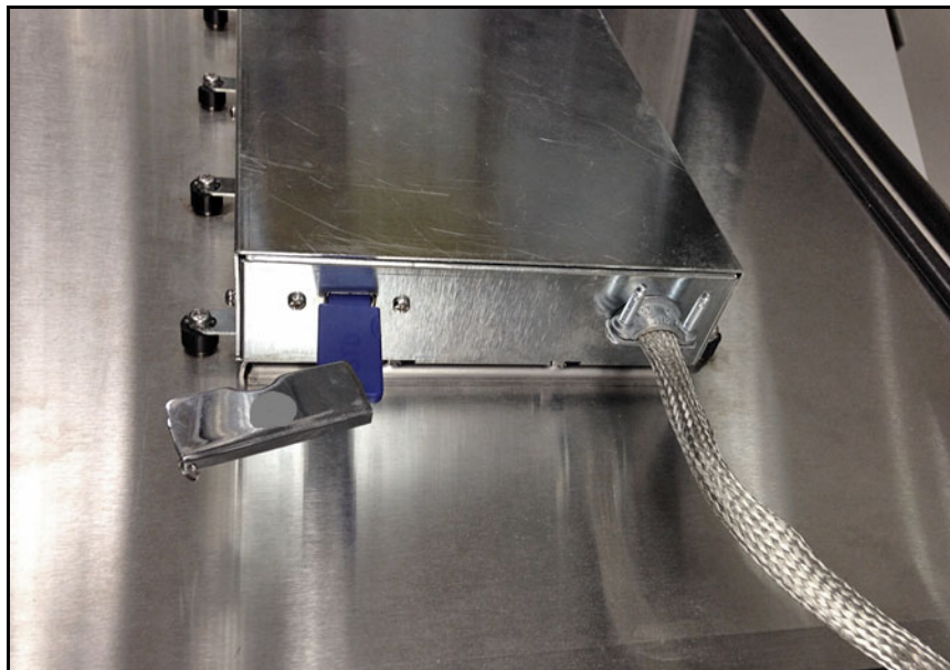
Figure 85: USB Flash Drive Plugged into Chassis Inside the Door
