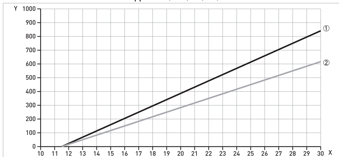
Figure 8-2: Non-Ex and Hazardous Location approval (Ex i / IS / NI): minimum power supply voltage for an output of 22 mA (switch output - relay option: 30 mA) at the terminals
