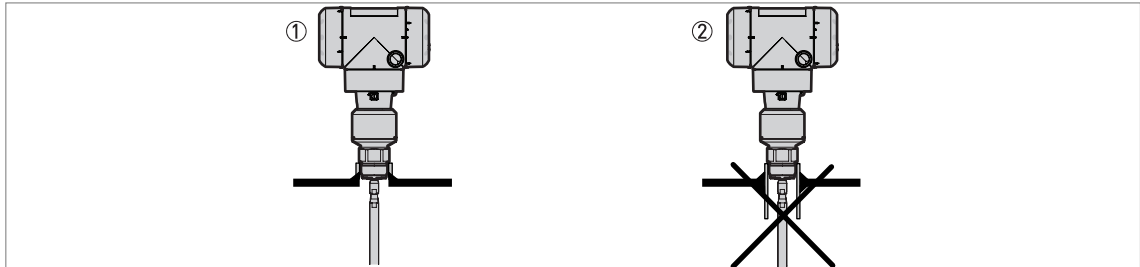
Figure 3-7: Sockets for threaded process connections
