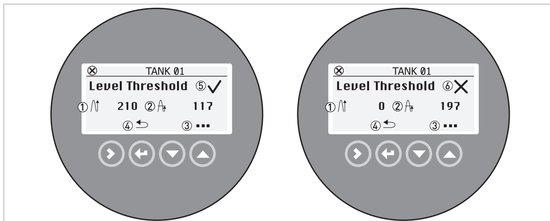
Figure 6-9: How to use thresholds (level signal and threshold data shown in this example)
