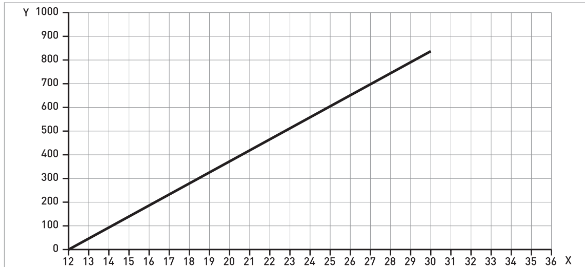
Figure 8-4: Minimum power supply voltage for an output of 21.5 mA at the terminal (Non-Ex and Hazardous Location approval (Ex i / IS))
