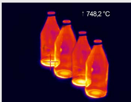
Hot-spot measurement in the production of glass bottles
