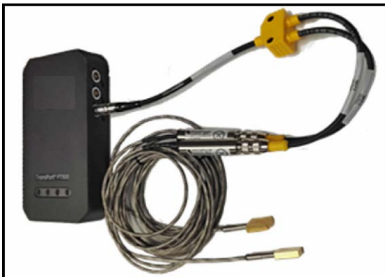
Figure 47: Energy Cable Connection (Right Side)
