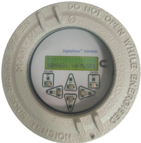
Figure 15: Display and magnetic keypad
