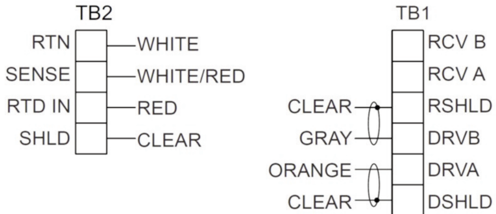
Figure 3-4: Wiring for Rosemount 56 and 1056 transmitters
