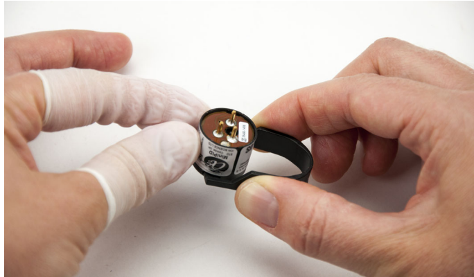
Figure 24: Using Removal Tool
