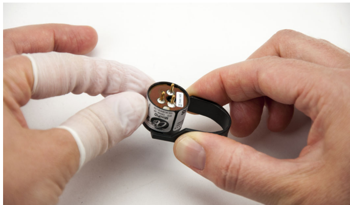
Figure 30: Using Removal Tool
