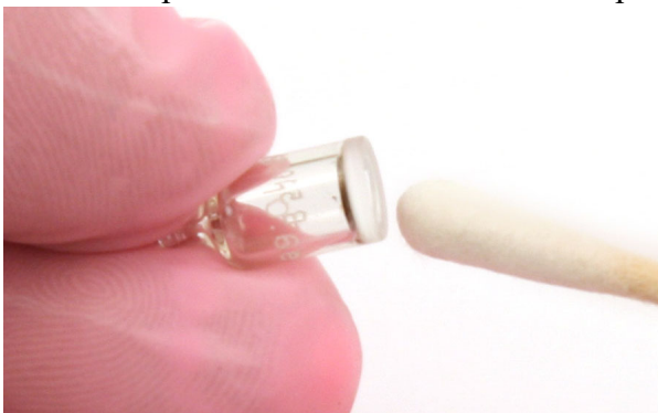
Figure 26: Polishing the Electrode Lamp Window
