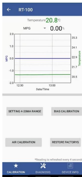
Figure 27. – Calibration Screen Interface uPyxis Mobile APP.
