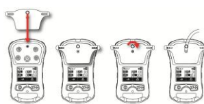
Install the calibration adapter on the QRAE 3 diffusion model
