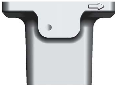
Figure 4. Flow Direction Arrow
