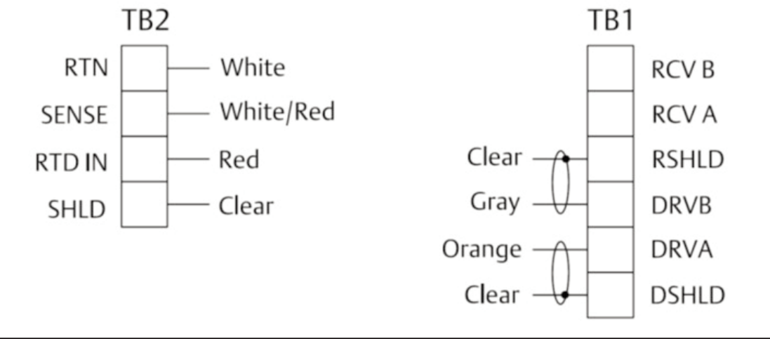
Figure 3-3: Rosemount 403/403VP Sensor Wiring to Rosemount 1066 Transmitter
