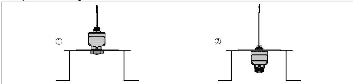
Figure 3-3: Installation of a device with a low-pressure flange (accessory)
