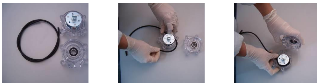
Figure 7.1: Pump tubing replacement.
