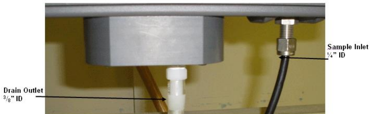
Figure 6 Bottom of the wet section case, with sample inlet and drain connections
