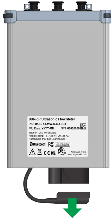
Figure 25: Slide battery pack out from handheld
