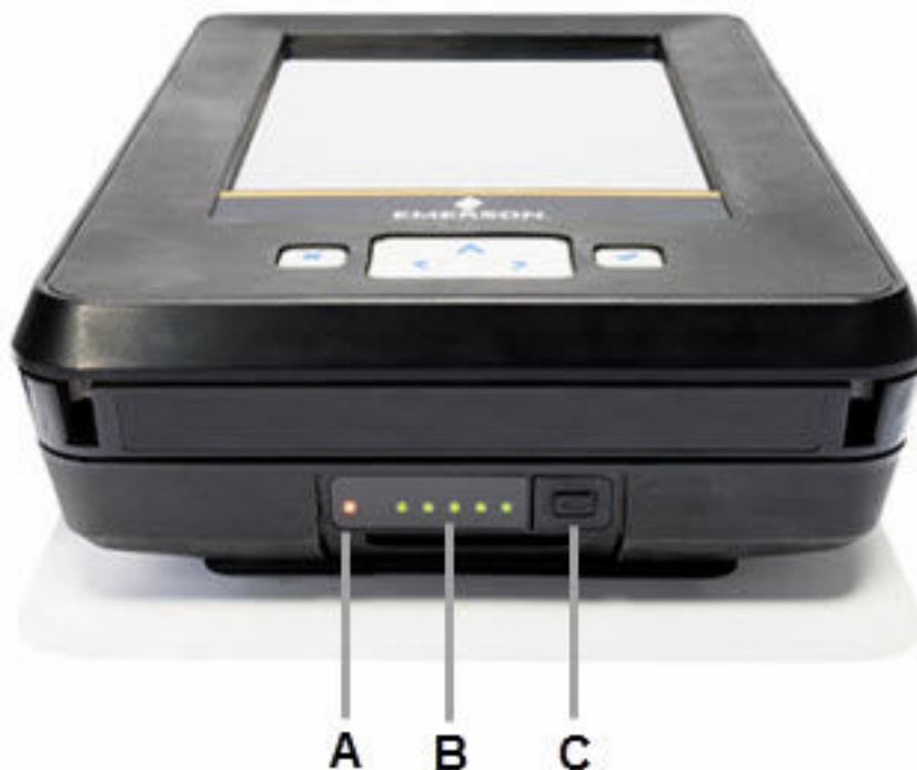
Figure 2-8: LEDs showing approximately 100 percent charge
