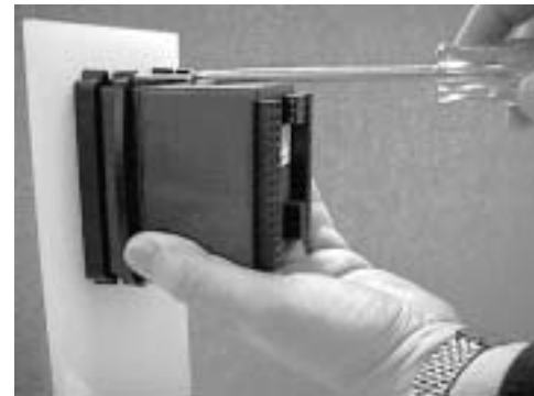
Figure 8.3c — Tightening the Screws.
