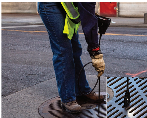
Figure 6.2 Insert the probe into the test area.
