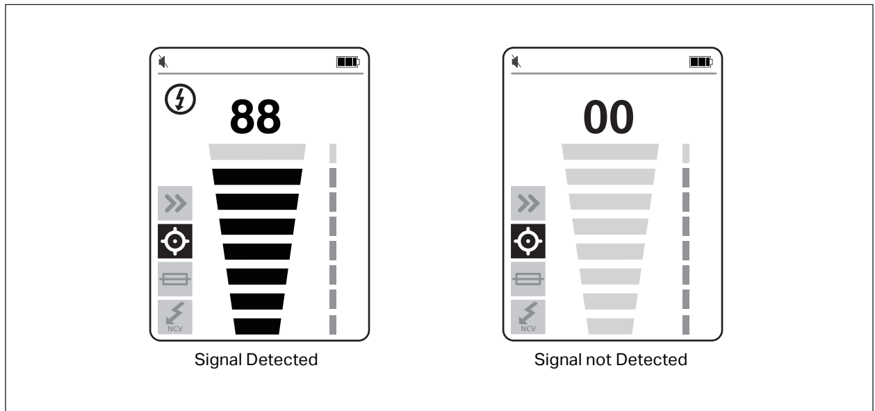
Figure 10. Tip Sensor Signal Strength (2052R)
