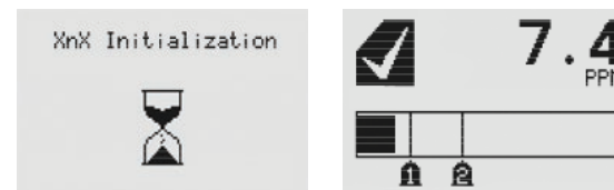
Figure 60. XNX Initialization and General Status screens
