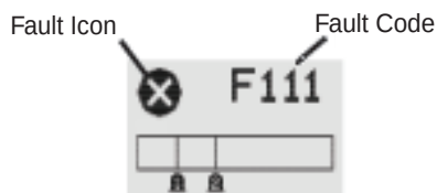
Figure 12. General Status Fault detail
