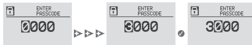
Figure 17. Entering the passcode
