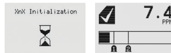
Figure 61. XNX Initialization and General Status screens
