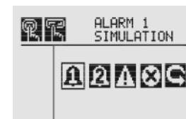
Figure 155. Alarm/Fault Simulation menu
