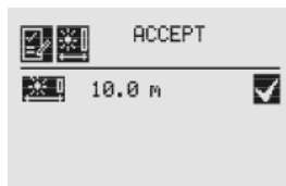
Figure 121. Accepting Path Length Changes
