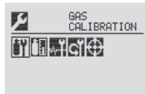
Figure 42. Gas Calibration menu
