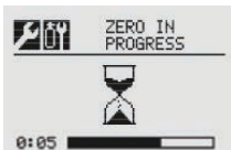
Figure 44. Zero Calibration in Progress
