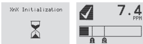
Figure 27. XNX Initialization and General Status screens
