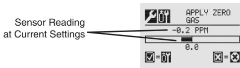
Figure 43. Zero Calibration screen
