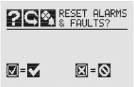
Figure 21. Alarm/Fault Reset Confirmation Screen
