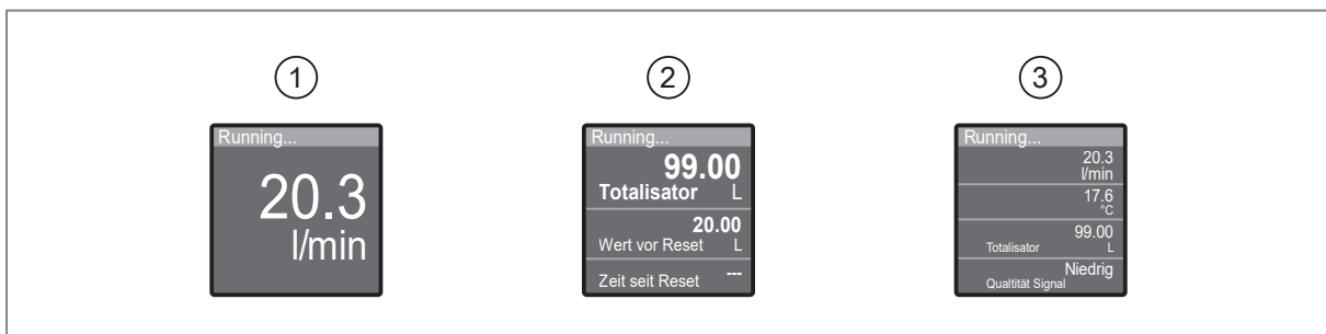
Fig. 21: Switching between the process value displays
