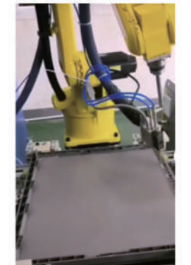
Control cabinet door panel gluing
