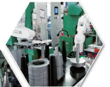
Motor stator silicon steel sheet handling
