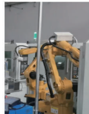
Island one-to-three machine loading and unloading
