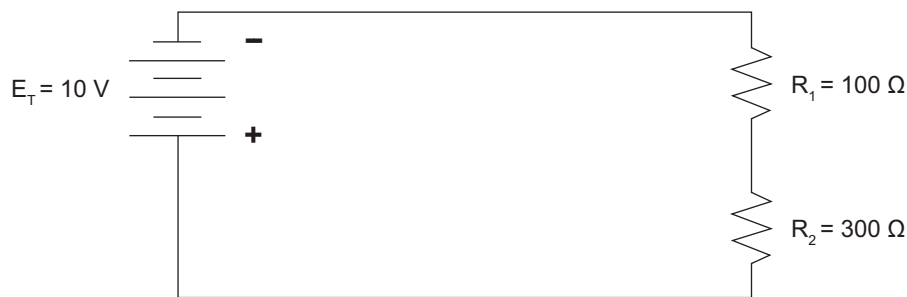
Figure 5-2. Series Resistive Circuit
