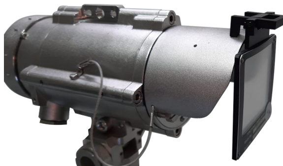
Figure 6-5: Detector with Functional Check Filter Installed
